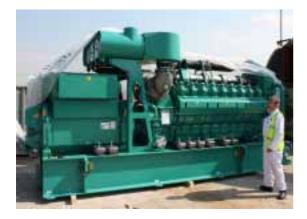
The huge units (at  $6.3 \times 2.1 \times 2.8$  metres each) were out of gauge, meaning they would not even fit, let alone load into a standard 40' container, so we had to use specialist open top containers for each generator.
